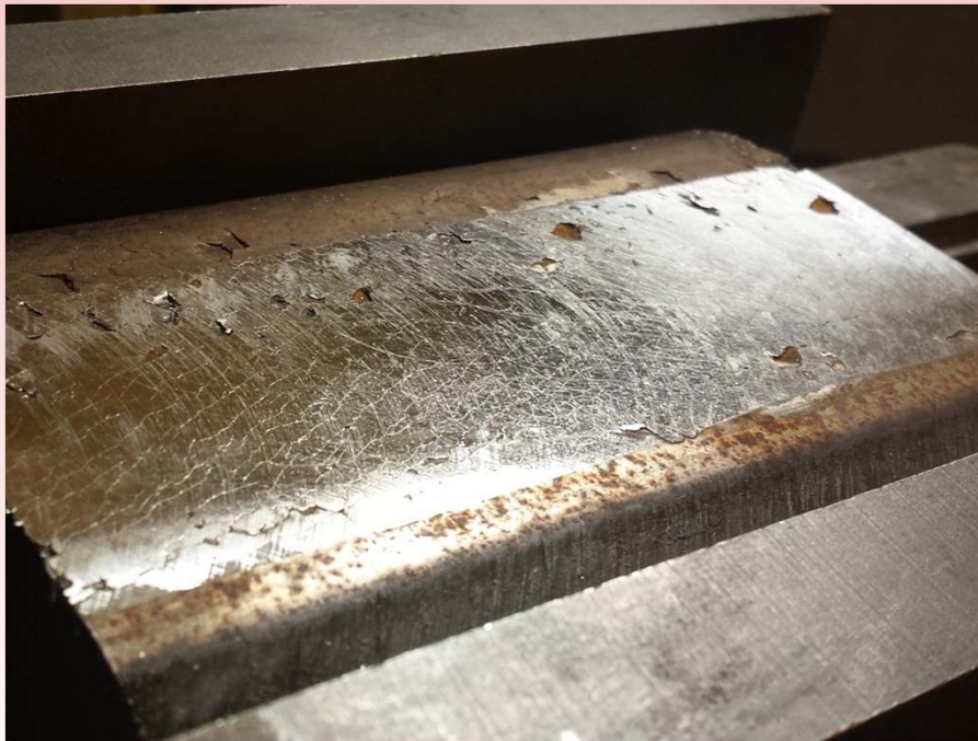
1 st pass, depth 0.5 mm (gage near)
