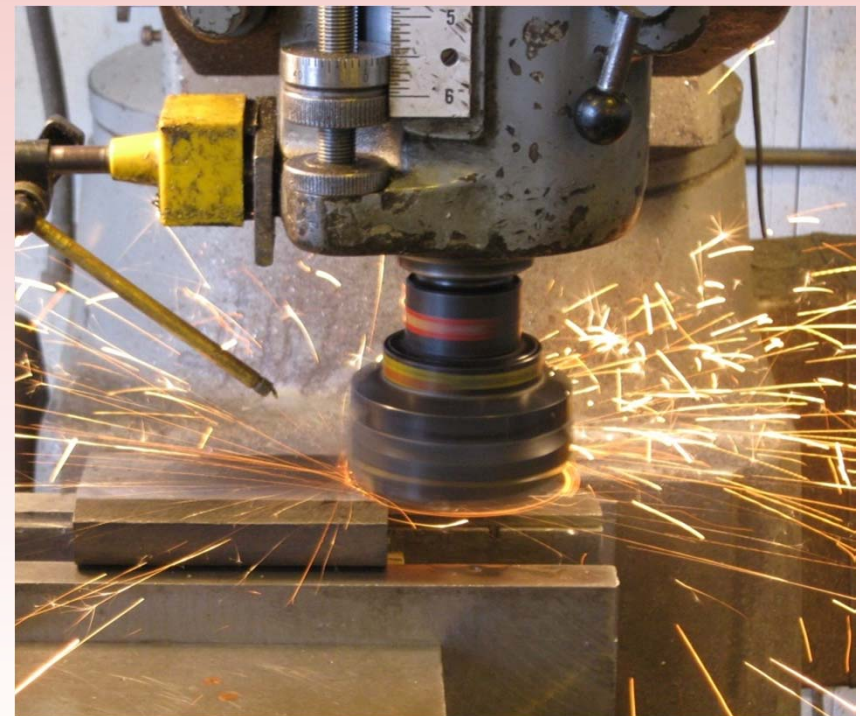
Rail head removal by milling
